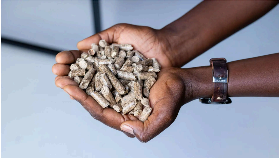
Figure 1: EcoMoto pellet briquette fuel made in Kenya from 100% waste biomass (Source: https://ecosafi.com/the-difference/ )
